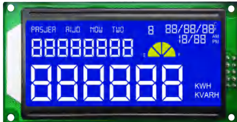
电力仪表显示屏
