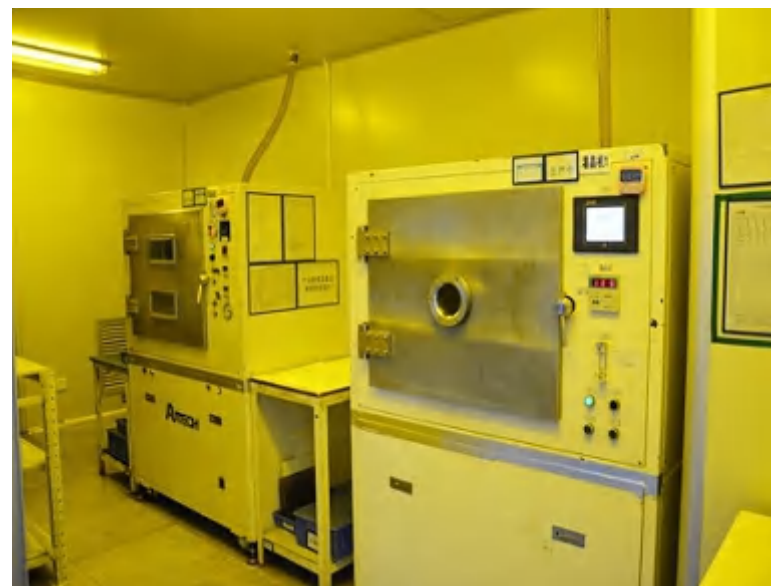
LCD灌晶工序/LCD Filling Process
