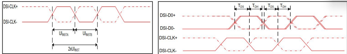
Figure 4 DSI clock channel timing
